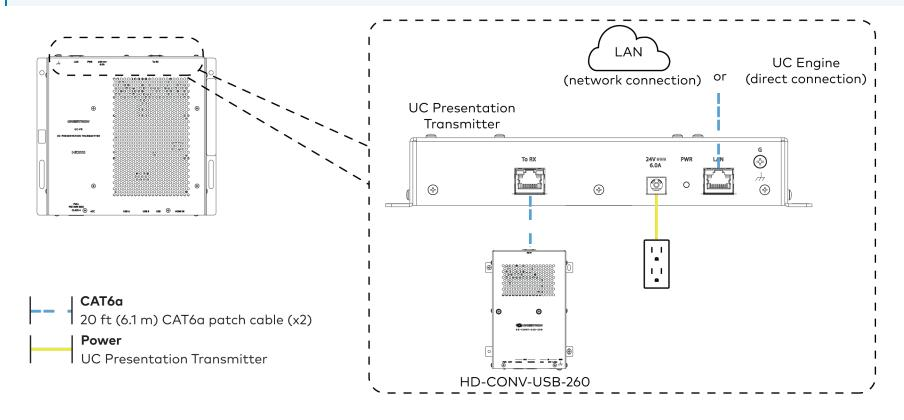
4. Connect the touch screen to the bottom of the UC Presentation Transmitter.
