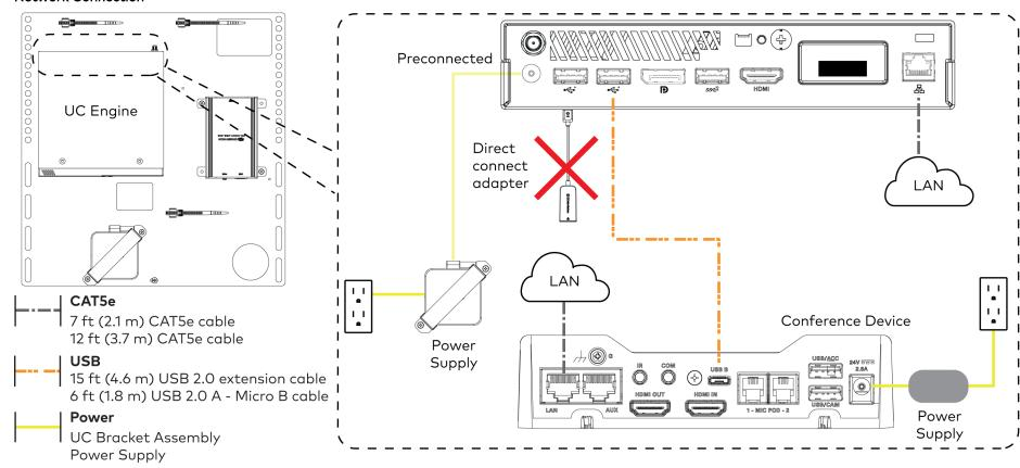
2. Connect displays to the UC Engine. Connect the EDID passthroughs to the displays.
