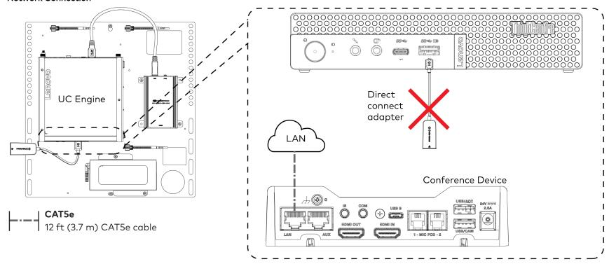
2. Make camera, conference device, and network connections to the top of the UC Engine. Connect the bracket assembly's integrated power supply and the conference device's power supply to AC power outlets.
