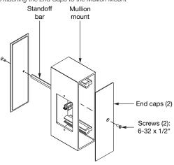
3. Connect the cable connector to the SSW's rear assembly, and then attach the assembly to the mullion mount's 1-gang opening using two 6-32 x 5/16" screws (included with the SSW) and a Phillips screwdriver (not included).
