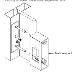
6. Secure the mullion mount to the toggle bolt rods with the metal locking plate. Use the included Allen wrench and the two 8-32 x 5/8" screws to attach the locking plate to the bolt rods.
