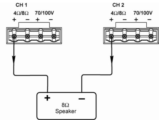
**NOTE:** The **INPUT LEVEL** controls for both channels must be set to the same level.
