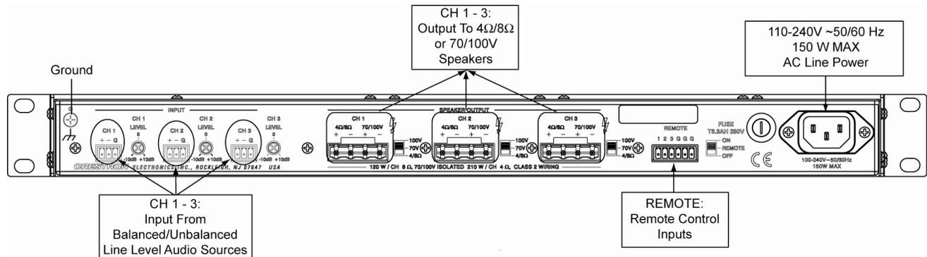
**NOTE:** Ensure the unit is properly grounded by connecting the chassis ground lug to an earth ground (building steel).
