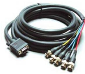
Kramer's C-GF/5BM graphics video breakout cable is constructed of 5 mini coax cables with a molded 15-pin HD (M or F) on one end and 5 BNC (M or F) on the other. It converts between the two most common cabling formats used for routing computer graphic video signals, 15-pin HD, and 5 BNC
