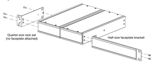
NOTE: Do not attach faceplates to rack ears that are attached to the length of the amplifier.
