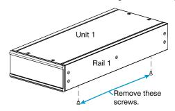
2. Remove rail 1 from unit 1 by sliding it off the side of the amplifier.
