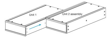
5. Secure unit 1 to the unit 2 assembly with the two screws removed in step 1.
