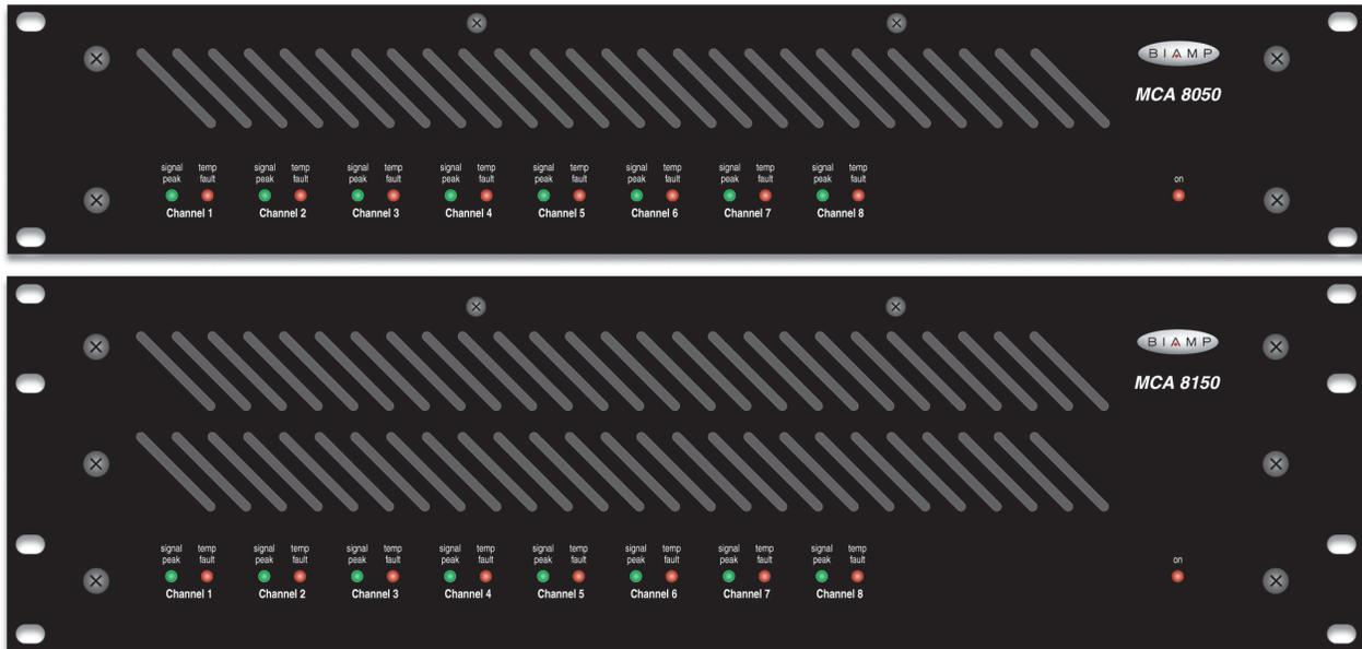
**MCA Series Multi-Channel Amplifiers provide eight channels of power amplification. Model MCA 8050 delivers 50 watts/channel into 4 ohms. Model MCA 8150 delivers 150 watts/channel into 4 ohms. Channels may be bridged in pairs for higher combined wattage. MCA Series amplifiers are covered by a five-year warranty.**
