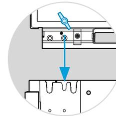
Look in from the sides of the screen to see the wing nut screws. The wing nut screws must enter the center slot on both sides of the screen.
