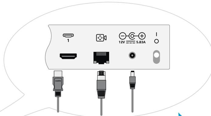
Check that the cables are not pinched when you tilt the camera back into normal position.
