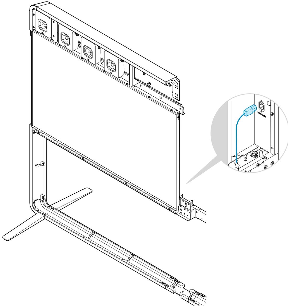
A power cable is attached to the right side of the screen. Connect it to the nearby connector.
