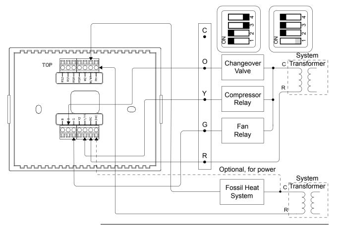
**NOTE:** The diagram above applies where furnace control is not integrated into the heat pump system.
