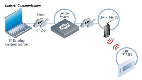
The CHV-TSTATEX connects to the CEN-RFGW-EX (gateway), which connects to control system via Ethernet, or the CHV-TSTATEX connects directly to an MC3 Control System.
