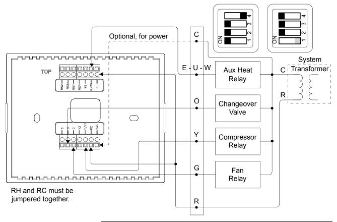
**NOTE:** Heat pump and dual-fuel heat pump systems require an outdoor temperature source (such as Crestron's CHV-RTS, sold separately) to function properly.
