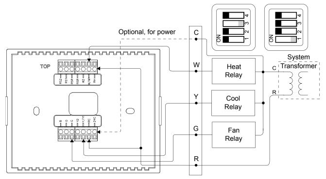
RH and RC must be jumpered together.
