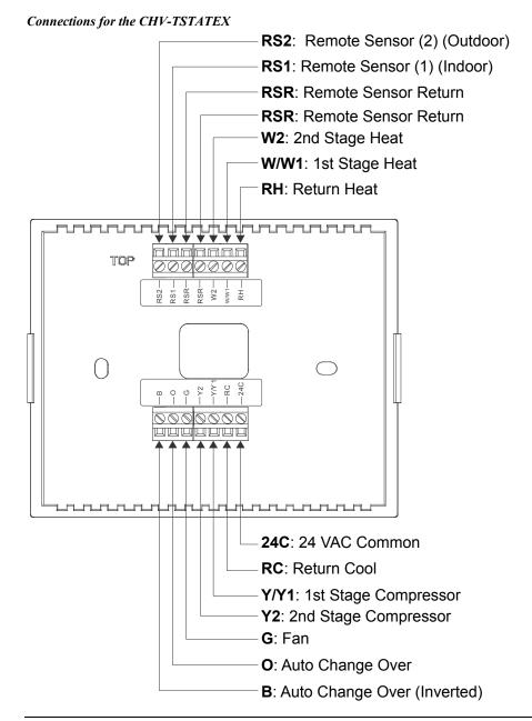
**NOTE:** 24 volt power is returned through the **RH** connector. Refer to wiring diagrams on the following pages.
