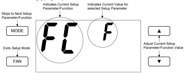
**NOTE:** When the CHV-TSTATEX is in *Setup* mode the large 7-segment displays show the current setup parameter/function. The small 7-segment displays show the current value for the selected setup parameter, if applicable, or it displays "—" when a function is selected. All other display elements are hidden (refer to "LCD Display" which starts on page 32).
