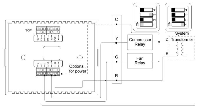
**NOTE:** A jumper wire must be placed between **RC** to **RH** for in order to provide power.
