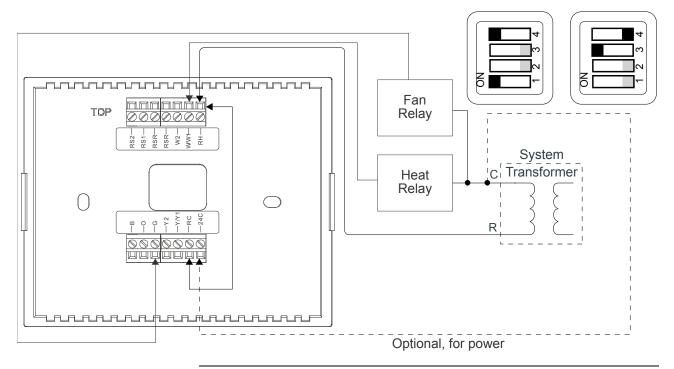
**NOTE:** To run fan during heat calls, be sure to enable the DIP switches. Refer to "DIP Switch Setup" which starts on page 11 for details.
