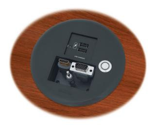
The Cable Cubby® 100 is a compact, round furniture-mountable cable access enclosure for AV connectivity and AC or USB power. Its convenient round design eliminates the need to measure or use a routing template, making installation quick and easy using a standard four inch hole saw. Its space-saving design is ideal for lecterns or any application where a single user access point is required.
