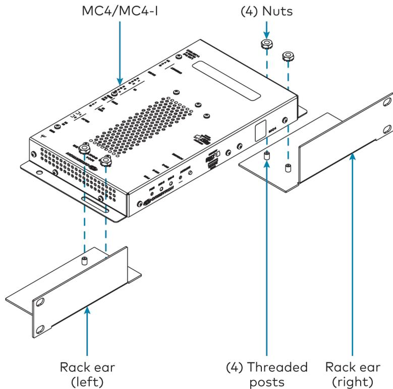
2. Secure the control system to the rack rails using four rack mounting screws (not provided).
