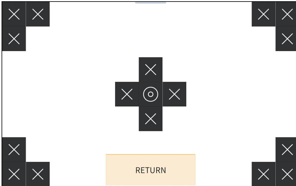
Use the touch test screen to test the touch functionality of the display. When a location button is tapped, its respective indicator lights on the screen.
