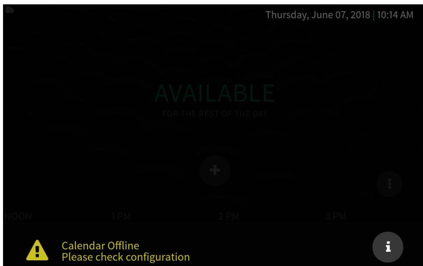
Place five fingers on the display and hold for 20 seconds to display the main Setup screen (TSS-770 shown).
