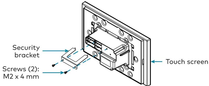
To remove the touch screen after installation, use the included release key to push down on the security bracket release tabs as shown in the following illustration while gently pulling the touch screen away from the mounting bracket.
