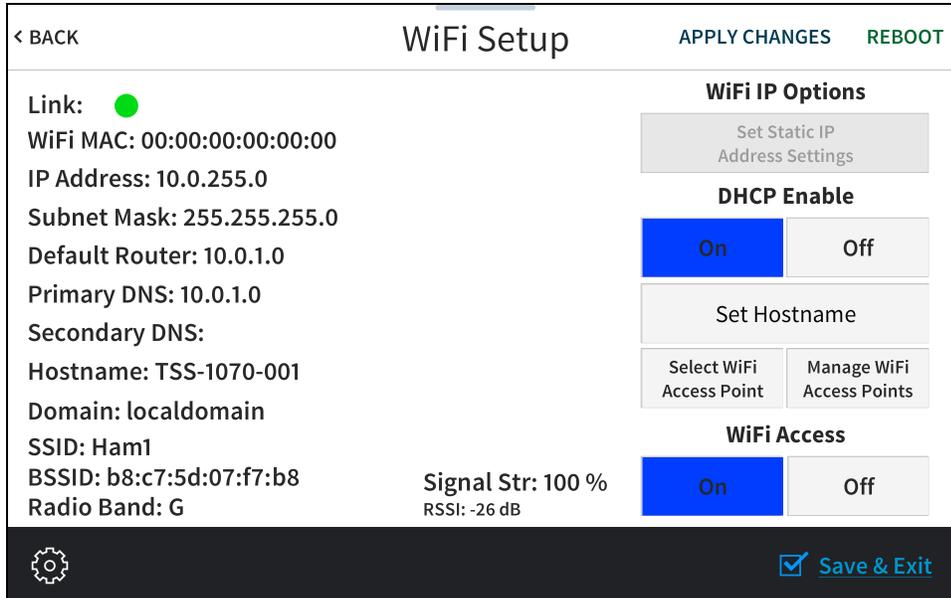
Use the Wi-Fi Setup screen to view the Wi-Fi network MAC and IP addresses, subnet mask address, default router address, primary and secondary DNS addresses, host name, domain, and various details about the Wi-Fi connection. A **Link** indicator is provided to indicate the status of the Wi-Fi connection. (Green indicates that the Wi-Fi connection is active.)
