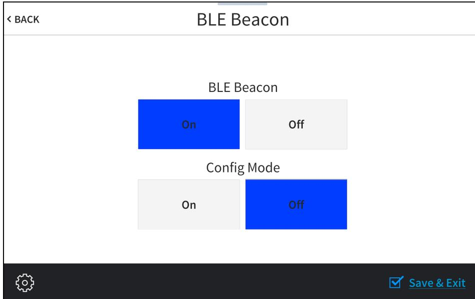
Use the **BLE Beacon** screen to configure the built-in PinPoint™ proximity detection beacon. Using Bluetooth® technology, the beacon works with the Crestron App or Crestron PinPoint App to determine when a mobile device is in or near the same room as the beacon, and signals the mobile app to automatically display the appropriate controls and information for the room.
