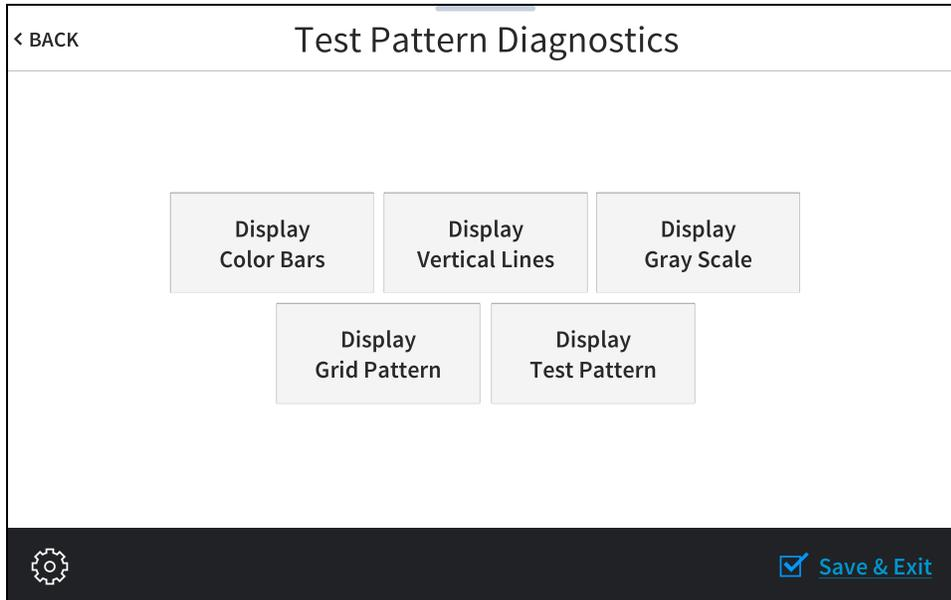
Use the **Test Pattern Diagnostics** screen to display any of the available test patterns. Tap one of the buttons on the screen to display its respective test pattern.
