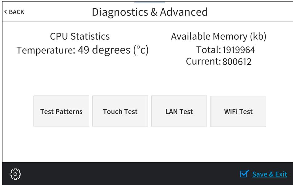
Use the **Diagnostics & Advanced** screen to access various diagnostic test screens for the touch screen. The **Diagnostics & Advanced** screen also provides the touch screen CPU temperature and available memory.
