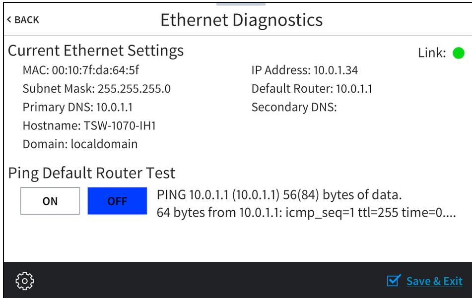
Use the **Ethernet Diagnostics** screen to view and test the Ethernet connection. The Ethernet Diagnostics screen displays the touch screen MAC and IP addresses, subnet mask address, default router address, primary and secondary DNS addresses, host name, and domain name. A **Link** indicator is provided to indicate the status of the Ethernet connection. (Green indicates that the Ethernet connection is active.)
