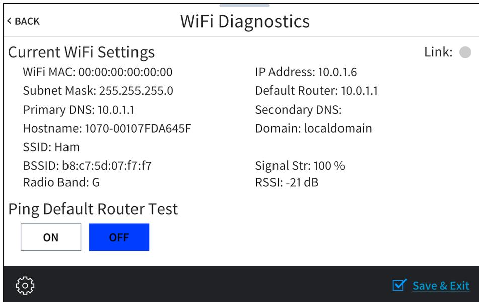
Use the **Wi-Fi Diagnostics** screen to view and test the Wi-Fi network connection. The Ethernet Diagnostics screen displays the Wi-Fi network MAC and IP addresses, subnet mask address, default router address, primary and secondary DNS addresses, host name, and domain name. A **Link** indicator is provided to indicate the status of the Wi-Fi network connection. (Green indicates that the Wi-Fi network connection is active.)
