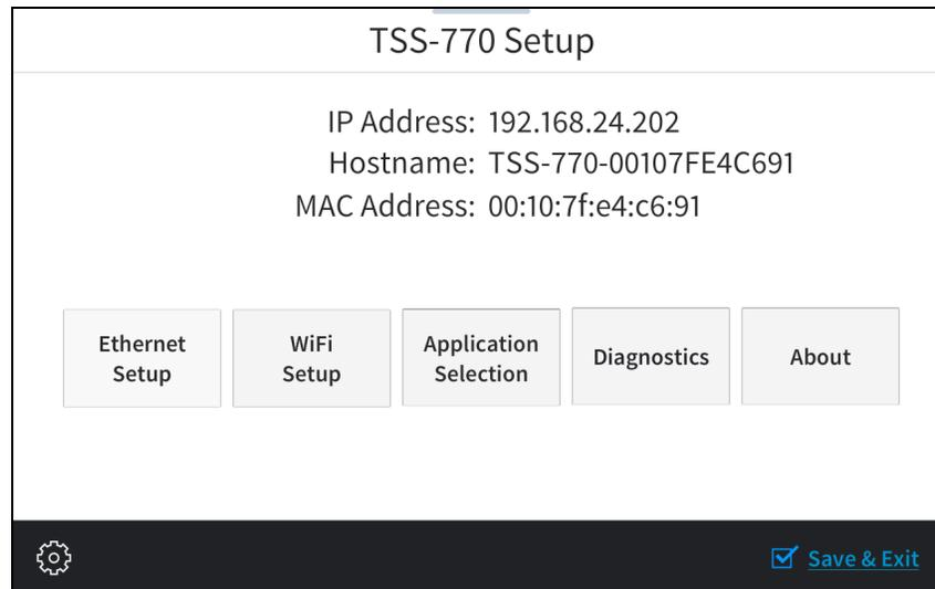
Use the setup screens to configure various settings for the touch screen, including Ethernet setup, scheduling application selection, Wi-Fi network setup, and diagnostics.
