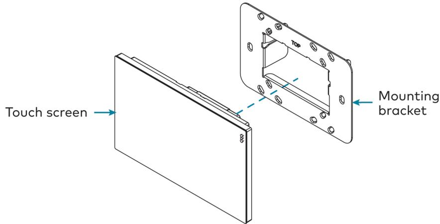
If the touch screen is not level after installation, pull it out of the mounting bracket and loosen the screws holding the bracket into place. This procedure allows the mounting bracket to be rotated slightly.
