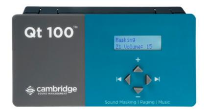
The Qt<sup>®</sup> 100 control module is a sound masking generator, controller and amplifier, with one auxiliary audio input to allow for distribution of audio from a paging controller or (background) music player. The Qt 100 control module is a compact one-zone controller suitable for installations of up to 12,000 square feet (1,115 m<sup>2</sup>). The masking level can be adjusted from the unit's front panel. Auxiliary audio level is set via the front panel.
