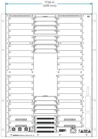
NOTE: Shown without input and output cards installed. All input and output cards sold separately.
