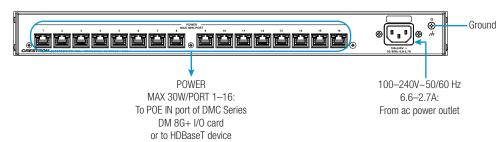
**NOTE:** Ensure that the device is properly grounded by connecting the chassis ground lug to an earth ground circuit (for example, building steel).
