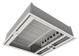
Fully finished enclosure designed to manage and store A/V equipment in an air handling plenum space above a NO or hard ceiling. These boxes are also equipped with the RackLink system, by Middle Atlantic Products. The box also has a built in projector mount that utilizes a 1 1/2" standard NFS fitting and is rated to support a load up to 50 lbs. The projector mount can move laterally and be positioned anywhere along the track.
