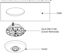
6. Align the arrows on the device with the arrows under the cover. Place the cover on the device and twist to secure. The cover snaps into place.
