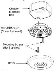
5. Align the arrows on the device with the arrows under the cover. Place the cover on the device and twist to secure. The cover snaps into place.
