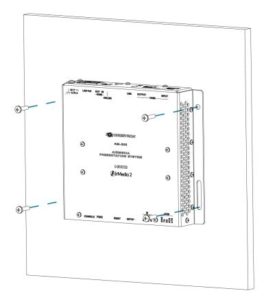
**NOTE:** The anchors are best suited for surfaces with 3/8 in. to 3/4 in. thickness.
